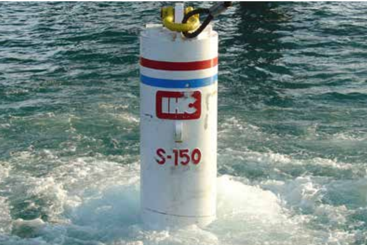
The Hydrohammer® can be driven at full energy in every thinkable position above and under water
